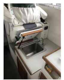
The sink is located under the captain's seat. A 30 gallon freshwater tank provides fresh water. Take care not to crush the spout when you lower the seat.
