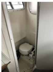
The marine head is a manual pump system with a holding tank, macerator, and dock pumpout fitting. The seawater inlet is valved and is located under the cabin floor. Do not put anything in the toilet except waste and marine toilet paper. You will be charged a steep fee if you plug the system with paper towels, home toilet paper, feminine products, or "flushable" wipes.
