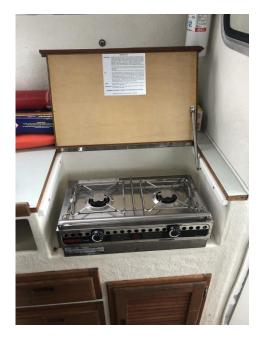
An alcohol fueled cook stove is offered in the galley. Take care when using it and watch for fires and CO. Do not use it as a heater when unattended. The user manual and additional fuel are onboard. Do not fill the stove through the burners, do not overfill, and follow the directions provided.
